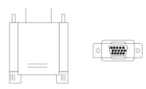
This motherboard has built in video facilities. Your monitor will attach directly to JVGA1 connector on the motherboard.
