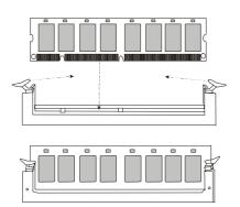
3. The Mounting Holes and plastic tabs should fit over the edge and hold the SDRAM DIMM memory modules in place.
