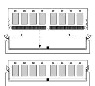
3. The Mounting Holes and plastic tabs should fit over the edge and hold the DDR DIMM memory modules in place.
